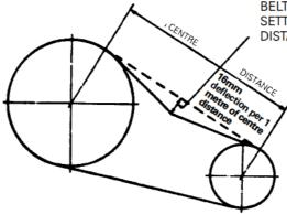
BELT TENSION INDICATOR APPLIES SETTING FORCE AT MID CENTRE DISTANCE
